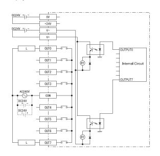
The I/O unit's power supply should be separated from Note: the sensor's power supply snound of Str. ... the sensor's power supply to prevent the unit from being affected by external noise.
