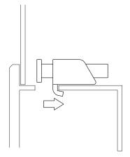
(4) Tighten the fastener screws equally in a diagonal pattern by using a Phillips screw driver. When tightening them, slowly increase the torque. (FP-3500T/3600T/3650T Series: 4 places, FP-3710T Series: 8 places, FP-3900T Series: 12 places)
