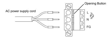
(4) After inserting all three pins, insert the Power Plug into the Power Connector at FP. Fix the plug with two(2) minus screws.
