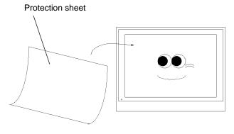
Attach the screen protection sheet when using the FP in extremely dirty or dusty areas.
