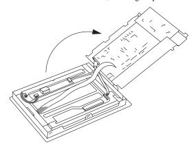
When the FP unit's power has just been turned OFF, the circuit board chassis is still very hot! Be sure to wear gloves to prevent being burned.
