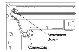
(6) Loose the backlight unit attachment screw. Next, slide the backlight in the direction shown and lift it forward and remove it from the FP.
