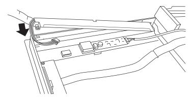
(8) Connect the backlight's one (1) power connector. Next, close the circuit board and secure the rear case in place using the attachment screws removed in steps 1), 2) and 3).
