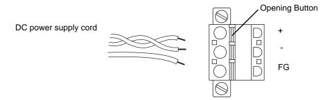
(4) After inserting all three pins, insert the Power Plug into the Power Connector at FP. Fix the plug with two(2) minus screws.
