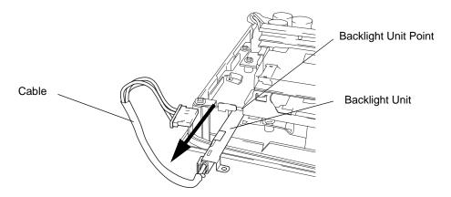
IMPORTANT | • The entire backlight unit should be changed, not just the backlight.
