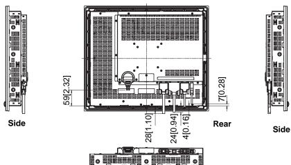
All the above values are designed in case of cable bending. The dimensions given here are representative values depending on the type of connection cable used. Therefore, they are all intended for reference only.
