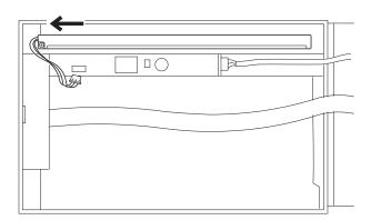
(7) Insert the new backlight in the FP. Insert the unit by sliding it in the direction shown in step 6).
