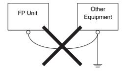
If this equipment does not function properly when grounded, disconnect the ground wire from the FG terminal.
