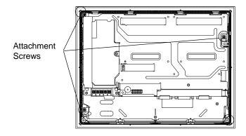
(4) The circuit board is connected on one side, and hinges open.
