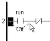
To create an automatic hold circuit, drag the "Run" circuit's left-side connection line to the right side to create an OR circuit. (see figure)
