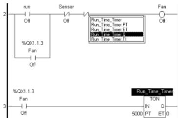
After "Run\_Time\_Timer" is dropped on Rung 2, a pop-up variable window will appear. Double-click on this window's [Run\_Time\_Timer.Q] variable, which designates the output bit used for "Run\_Time\_Timer."
