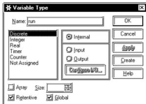
Enter "Run" in the "Name" field and select "Discrete" to specify the type of bit variable. Next, select "Internal" to specify that the variable being created is an internal variable, and click on [OK].
