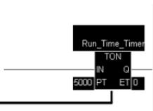
Use the same procedure to drag the On-delay Timer (Rung 2) to the base screen. The On-delay timer is treated as a Keypad Input Display when it is placed on a base screen.
