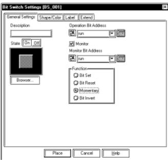
In the [Bit Switch Settings] dialog box, select "Momentary" in the "Function" area, which turns a bit (switch) ON only while the touch panel switch is touched. Next, click [Place] and position the bit switch on the base screen. The switch's label (text displayed on the switch) and shape can also be set.
