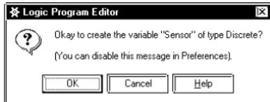
Click the [OK] button. Naming I3 creates a variable name for I3, and allocates that variable to the FN-XY08TS unit's No. 3 input terminal.
