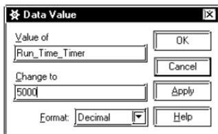
Double-click the "0" that appears in the lower left corner of the On-Delay timer to call up the [Data Value] dialog box. Enter "5000" (milliseconds) in the "Change to" field to set the operating time to five seconds, and click [OK].
