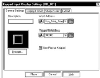
In the [Keypad Input Display Setting] dialog box, designate [Use Pop-up Keypad]. Next, click [Place] and position the Keypad Input Display on the base screen.
