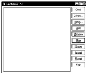
Here, to assign the variable names [Sensor] and [Fan] to external I/O, first, click the [Data] menu's [Configure I/O] selection. The [Configure I/O] window will then appear. Next, click the [Drivers] button and the following [I/O Drivers] dialog box will appear.
