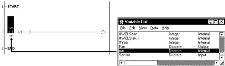
In Pro-Control's [Data] menu, click [Variable List]. From the list of variables, select "Run". Without releasing your mouse button, drag and drop "Run" to the far left side Normally-Open contact.
