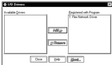
Select the Flex Network Driver listed in the GLC I/O list (left side), click the [Add] button, and click the [Close] button. The Configure I/O screen will then appear.
