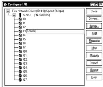
Under the FN-XY08TS, I0 through I7 and Q0 through Q7 are displayed. The "I" represents input, and the "Q" represents the output signal's external I/O. Here, double-click "I3", type "Sensor" and press [ENTER].
