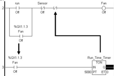
Drag the variable name "Fan" from Rung 2 and drop it onto the Normally-open contact in Rung 3.
