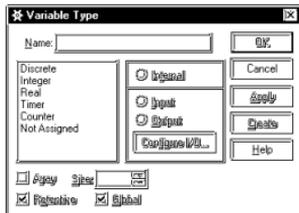
Here, we will create the variable "Run", which will correspond to an internal relay. First, in the Pro-Control Editor [Data] menu click [Variable Type] to call up the [Variable Type] dialog box.
