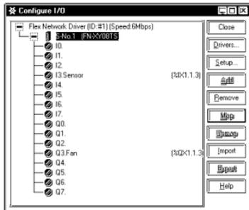
Next, use the same procedure to assign the name "Fan" to "Q3". Variable names allocated here are used by the logic program and/or screen creation software to access external devices. Here, the variable name "Sensor" stands for input from the sensor, and "Fan" for output sent to the fan.
