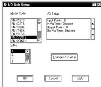
In the I/O Unit Setup screen's [Model Code] selection box, click on [FN-XY08TS] and click on [OK]. Control then returns to the Configure I/O screen.
